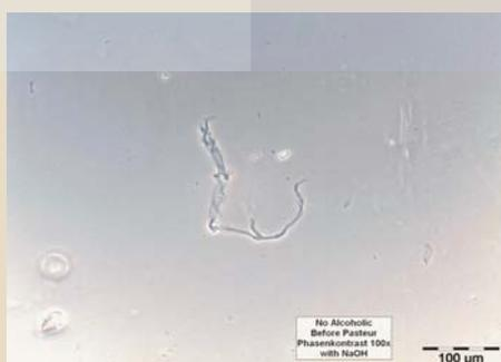
Fig. 7 Particles before tunnel pasteurization, after treatment with NaOH
