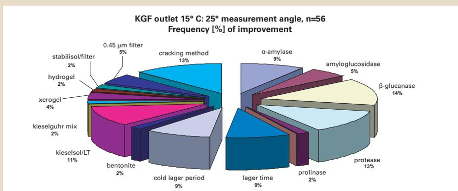
Fig. 2 Success rate of improvement measures for turbidity problems (measurement angle: 25°)
