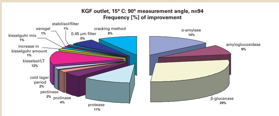
Fig. 1 Success rate of improvement measures for turbidity problems (measurement angle: 90°)
