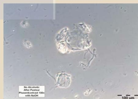
Fig. 8 Particles after tunnel pasteurization and treatment with NaOH
